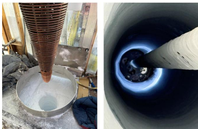
Left: the heated firn drill positioned over the pilot hole, right: the firn hole at around 15 meters depth (illuminated with a flashlight on a rope).
